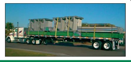
ONE TRUCKLOAD SHIPMENT CAN PROVIDE 10,000 SQ.FT. OF THE COMPLETE AL-SPEED<sup>®</sup> SHORING SYSTEM. SINGLE STAGE, UP TO 12" THICK SLAB.
