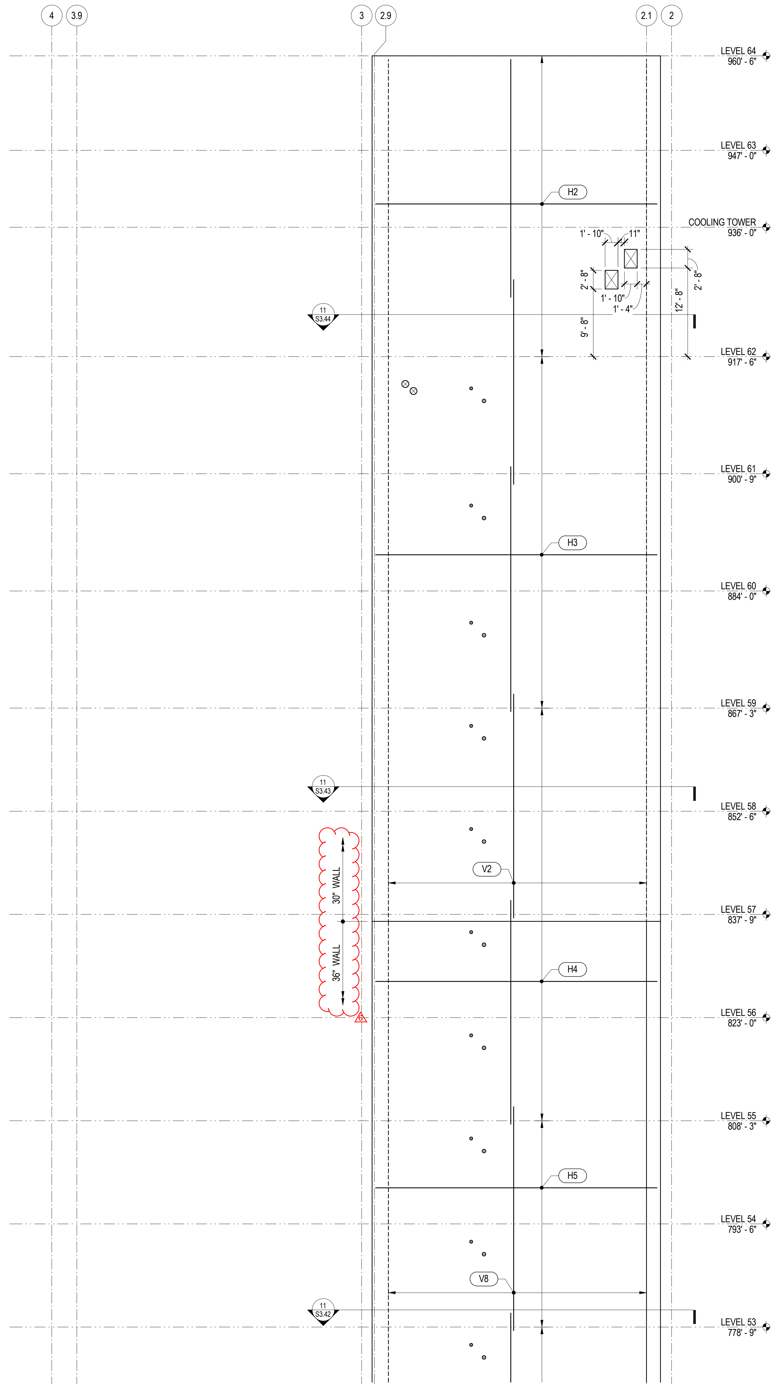
1 SHEAR WALL ELEVATION - WEST 1/8" = 1'-0"
