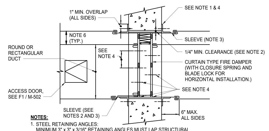
MINIMUM 3" x 3" x 3/16" RETAINING ANGLES MUST LAP STRUCTURAL OPENING 1" MINIMUM AND COVER CORNERS OF OPENINGS.
