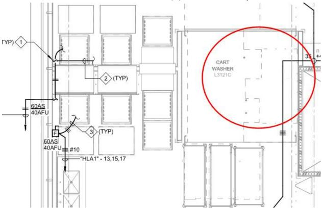
**f. Telecommuncation Plans:** The network port is not shown on the telecom drawings. We should make a note of this in the MEP Equipment Constructability Review Table.
