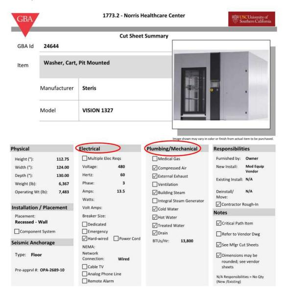
c. **Mechanical Plans:** No external exhaust is shown on the mechanical plans, but the building steam is shown (see highlight). We should make a note of this in the MEP Equipment Constructability Review Table.
