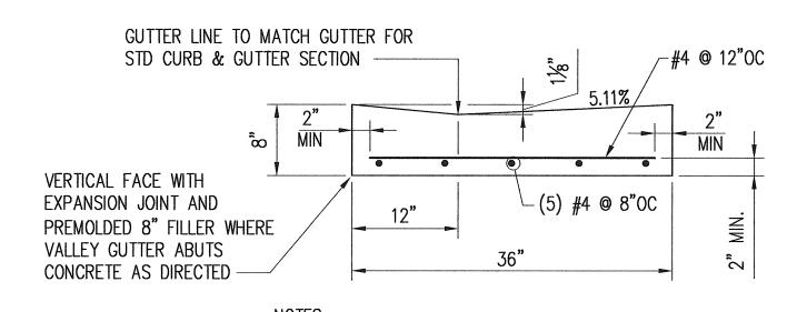
1. THE CONCRETE SHALL BE A MINIMUM OF CLASS 3000.
