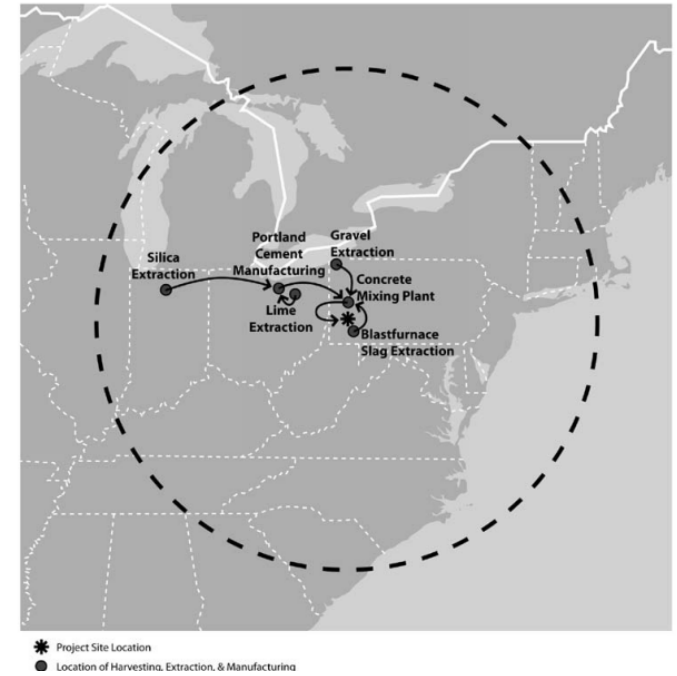
Figure 2. Extraction and Manufacturing Location of Fly Ash Concrete
