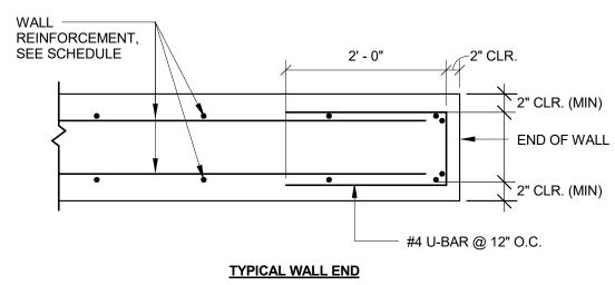
7 TYP. WALL COLUMN AND END ADD'L REINFORCING 3/4" = 1'-0"
