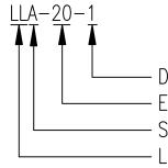
DAMPER NUMBER ELECTRIC CIRCUIT NUMBER SMOKE COMPARTMENT LEVEL
