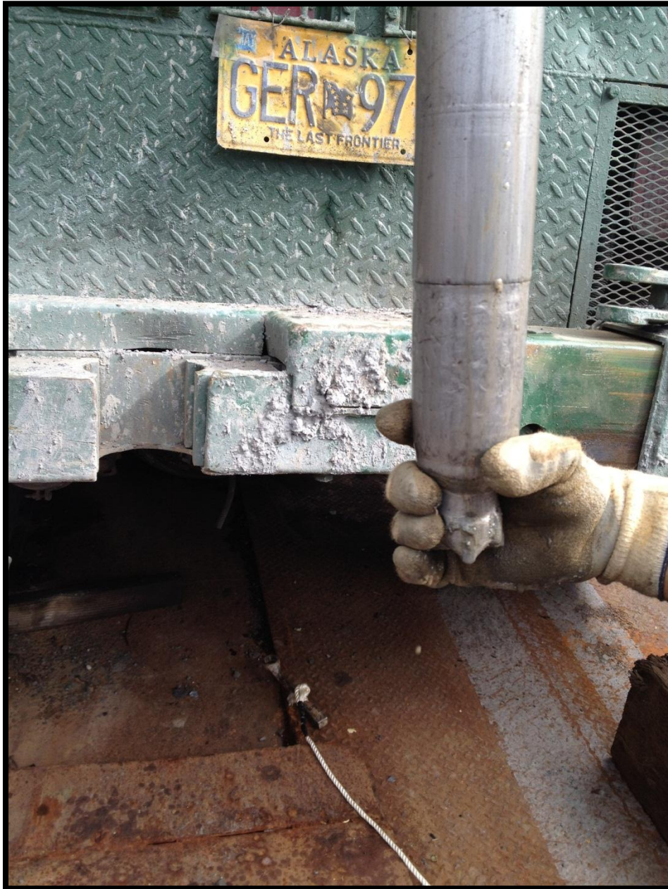
Blunt tip used on modified penetrometer (TH12-06)
