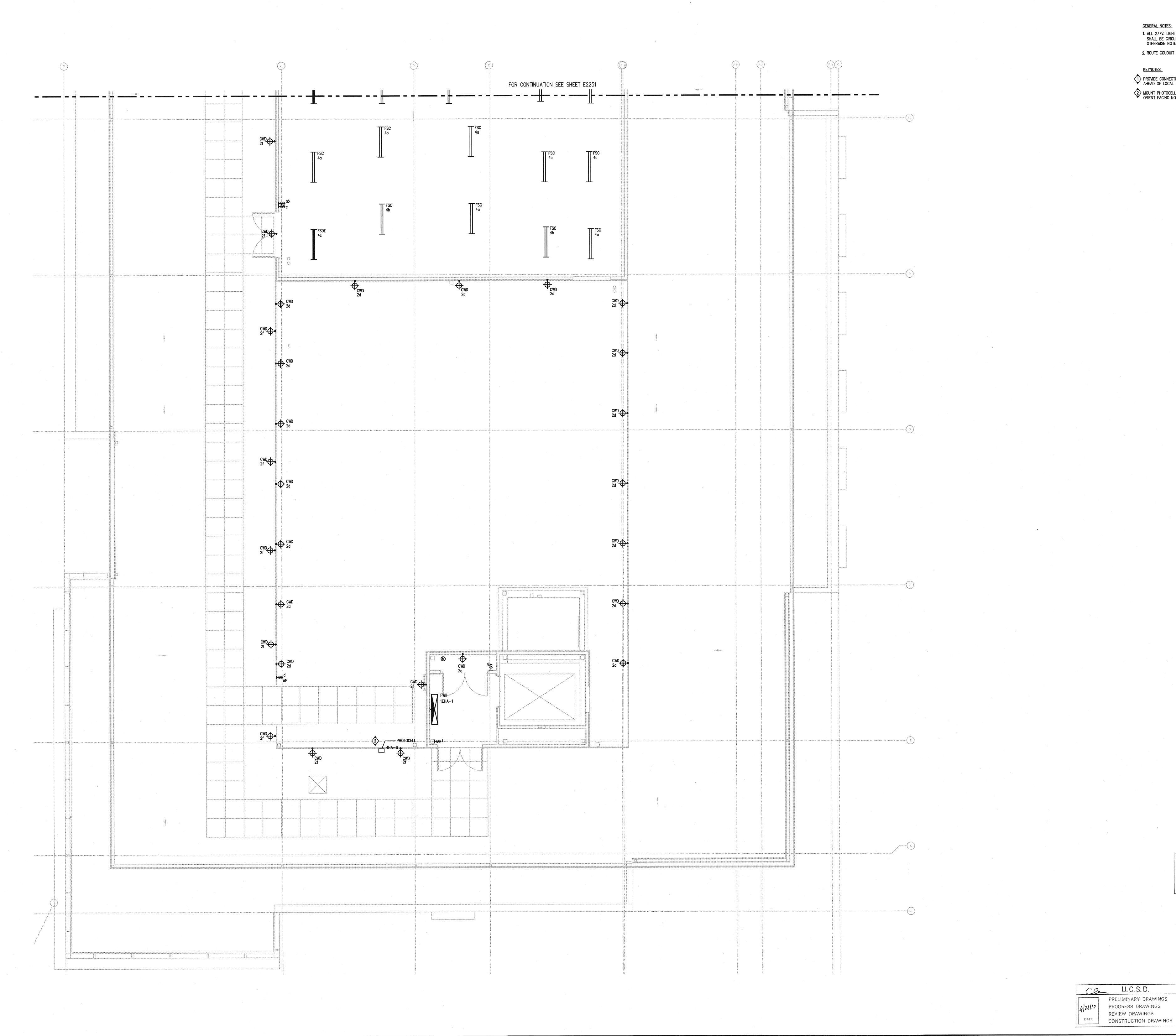
**GENERAL NOTES:** 1. ALL 277V. LIGHT FIXTURES ON THE ROOF SHALL BE CIRCUITED TO PANEL "4HA" UNLESS OTHERWISE NOTED. CIRCUIT NUMBER INDICATED. COPYRIGHT © FENTRESS ARCHITECTS
