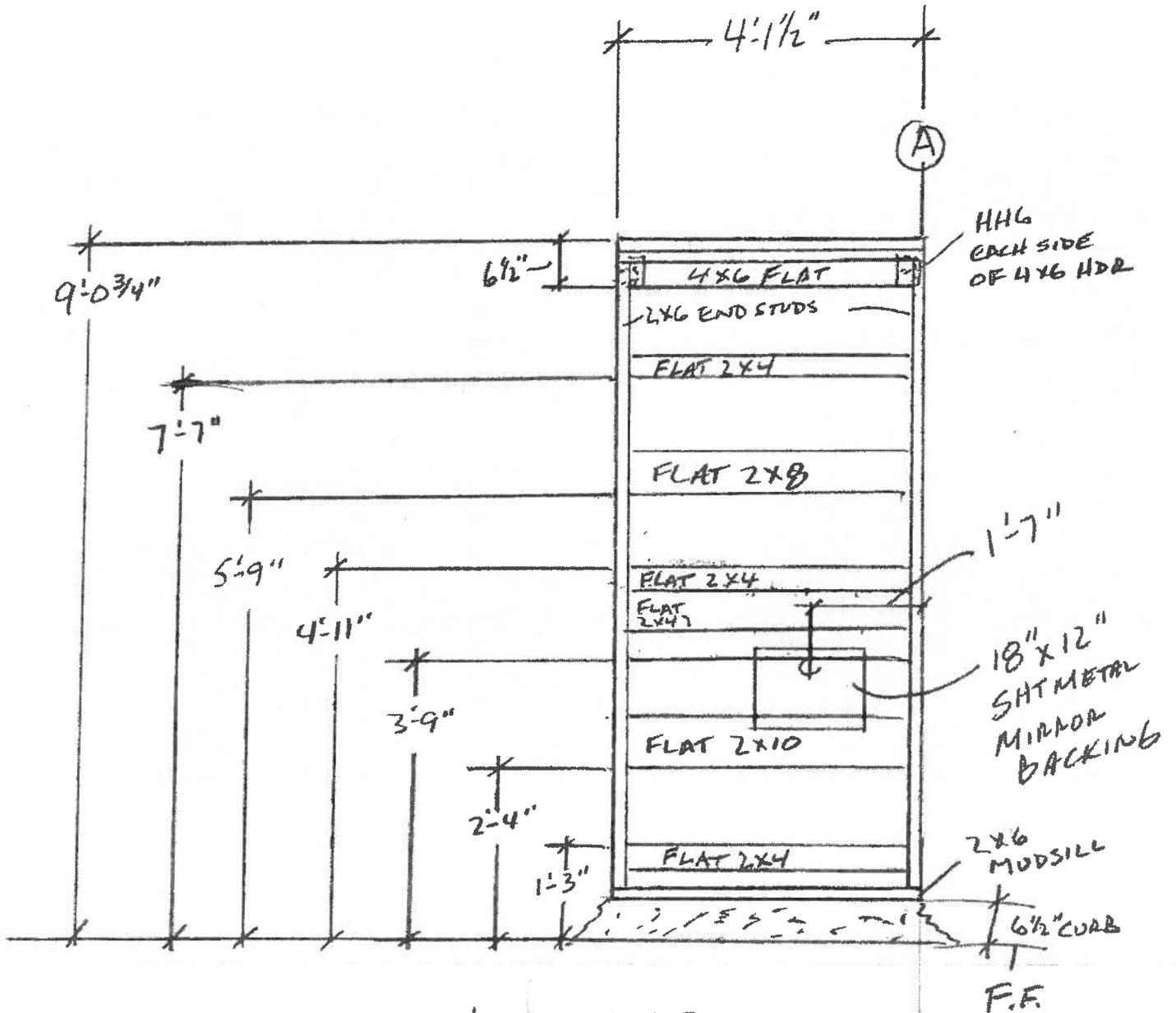
NOTE: FLAT 2X'S OCCUR AT BOTH SIDES OF WALL
