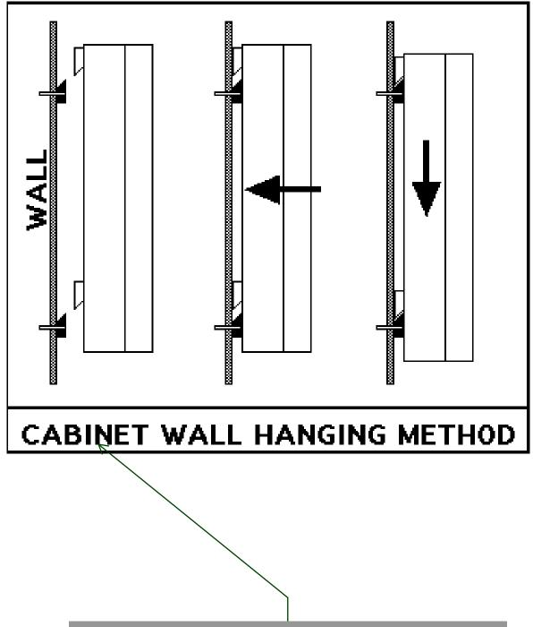
ROLLUDA please confirm that it is acceptable to install the top cabinets with the above wall cleat method, in lieu of standard in wall backing.
