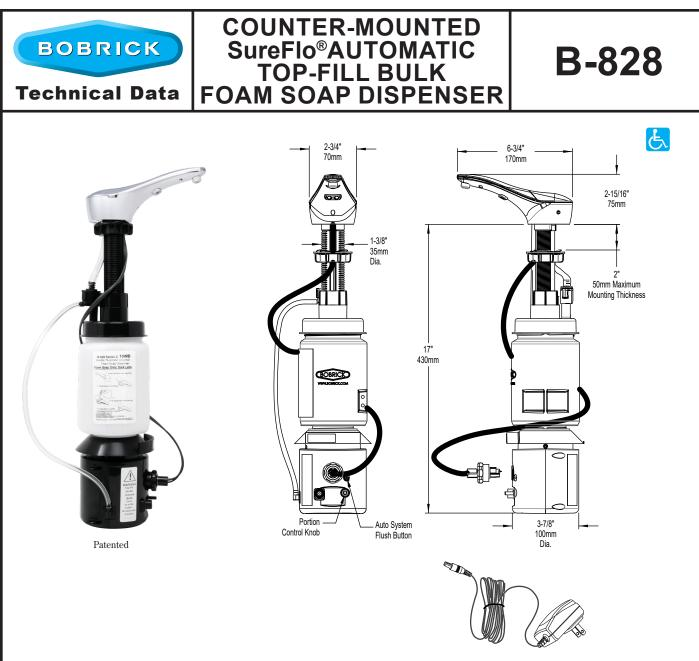
**Spout and Stem Assembly** — Above the counter, chrome plated ABS plastic spout. Unit is equipped with a spring loaded 180° rotatable lid with concealed locking mechanism for top filling. Rotatable lid mechanism consists of metal components. Integrated to Spout are a grey plastic Dispense Tip and Activation Lens Housing. Stem connects to Bottle.
