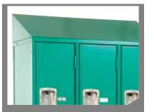
SLOPED TOPS - Sloped Tops prevent accumulation of books, clothes and other materials on top of lockers. DeBourgh constructs the 18-gauge slope top as a separate unit from the locker. This allows the lockers to be moved into a recessed area at a later time if desired. The slope top is attached at the factory with tamper proof fasteners, which reduces installation time.
