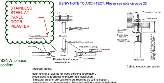
Wood support is not acceptable. Structural ceiling support and drilling for studs by others. Studs supplied by Hadrian but installed by others.
