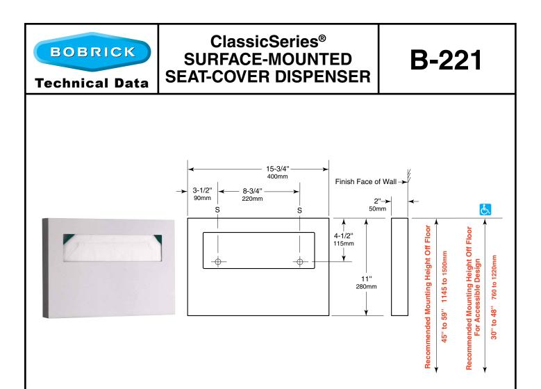
18-8, type-304, 22-gauge (0.8mm) stainless steel with satin finish. All-welded construction with beveled opening.
