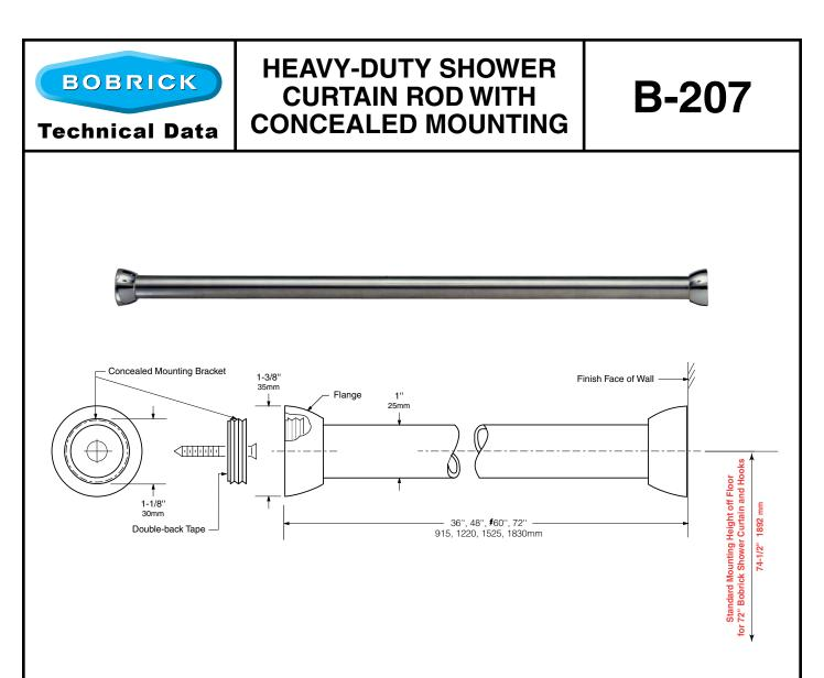
**Curtain Rod** — 18-8, Type-304, 20-gauge (1.0mm) stainless steel tubing with satin finish. 1" (25mm) outside diameter. Available in lengths from 36" (915mm) up to 72" (1830mm).
