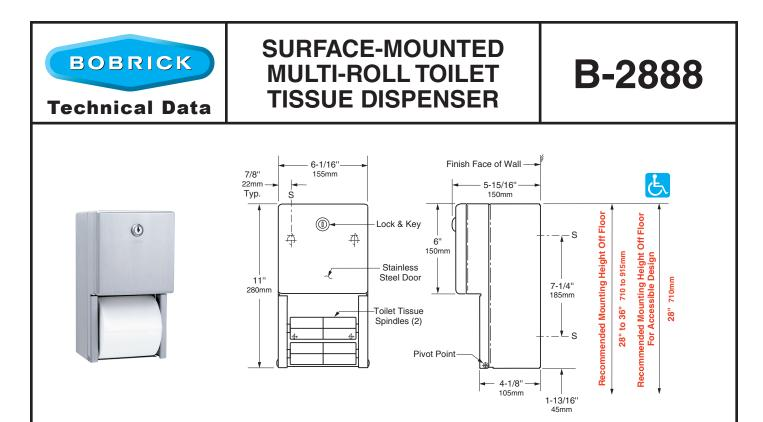
Cabinet — 18-8, type-304, 22-gauge (0.8mm) stainless steel. All-welded construction. Exposed surfaces have satin finish.
