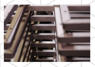
Slit steel mesh can be used for maximum ventilation and visibility due to the rigid structure of the angle steel.
