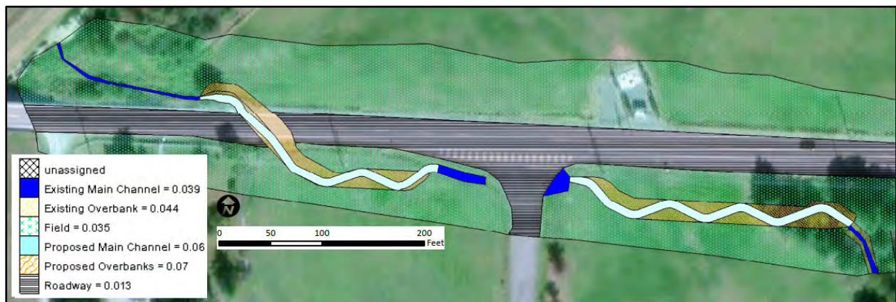
Figure 7.3. Spatial Distribution of Proposed-conditions Roughness Values in SRH-2D Model
