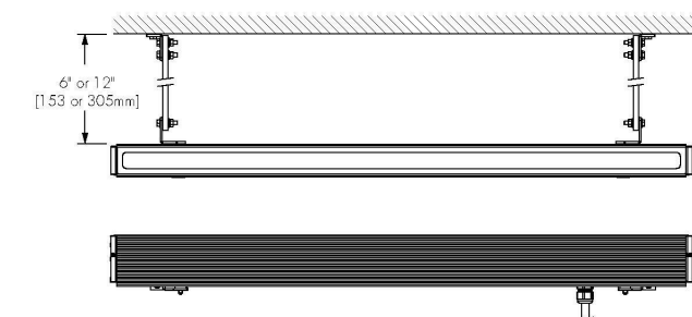
WAM6 & WAM12 Adjustable Extended Arm Mounting
