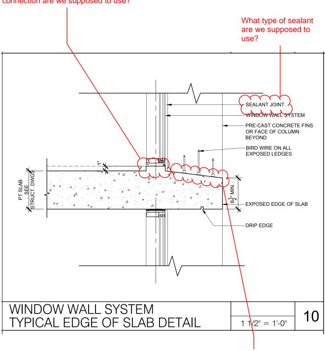
Need caulk joint between fin and slab for construction tolerance.
